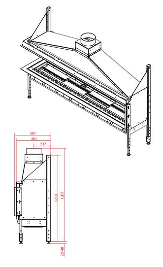
Fuel type - G20 (NG - 20mbar) Maximal gas rate- ~2,09 m Heat input (Hi)- ~19,74 kW
