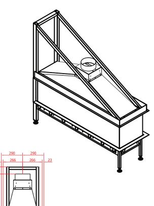
Fuel type - G20 (NG - 20mbar) Maximal gas rate- ~2,09 m³/h Heat input (Hi)- ~19,74 kW
