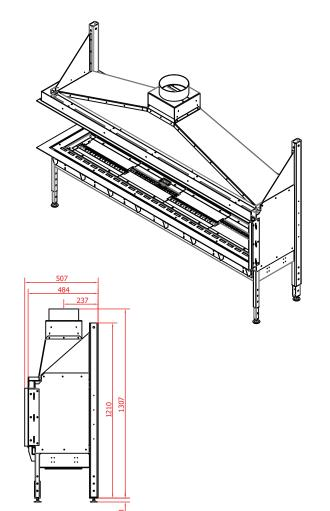
Fuel type - G20 (NG - 20mbar) Maximal gas rate- ~2,09 m Heat input (Hi)- ~19,74 kW
