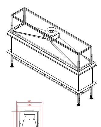
Fuel type - G20 (NG - 20mbar) Maximal gas rate- ~2,09 m³/h Heat input (Hi)- ~19,74 kW
