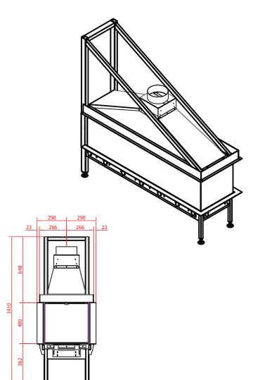
Fuel type - G31/30 (LPG - 37mbar) Maximal gas rate- ~1,13 kg/h Heat input (Hi)- ~14,26 kW
